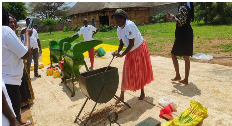
Figure 6: A private sector actor dealing in PHM equipment demonstrating the use of fabricated manual groundnuts sheller to the participants during PHM TOT in Moroto;
